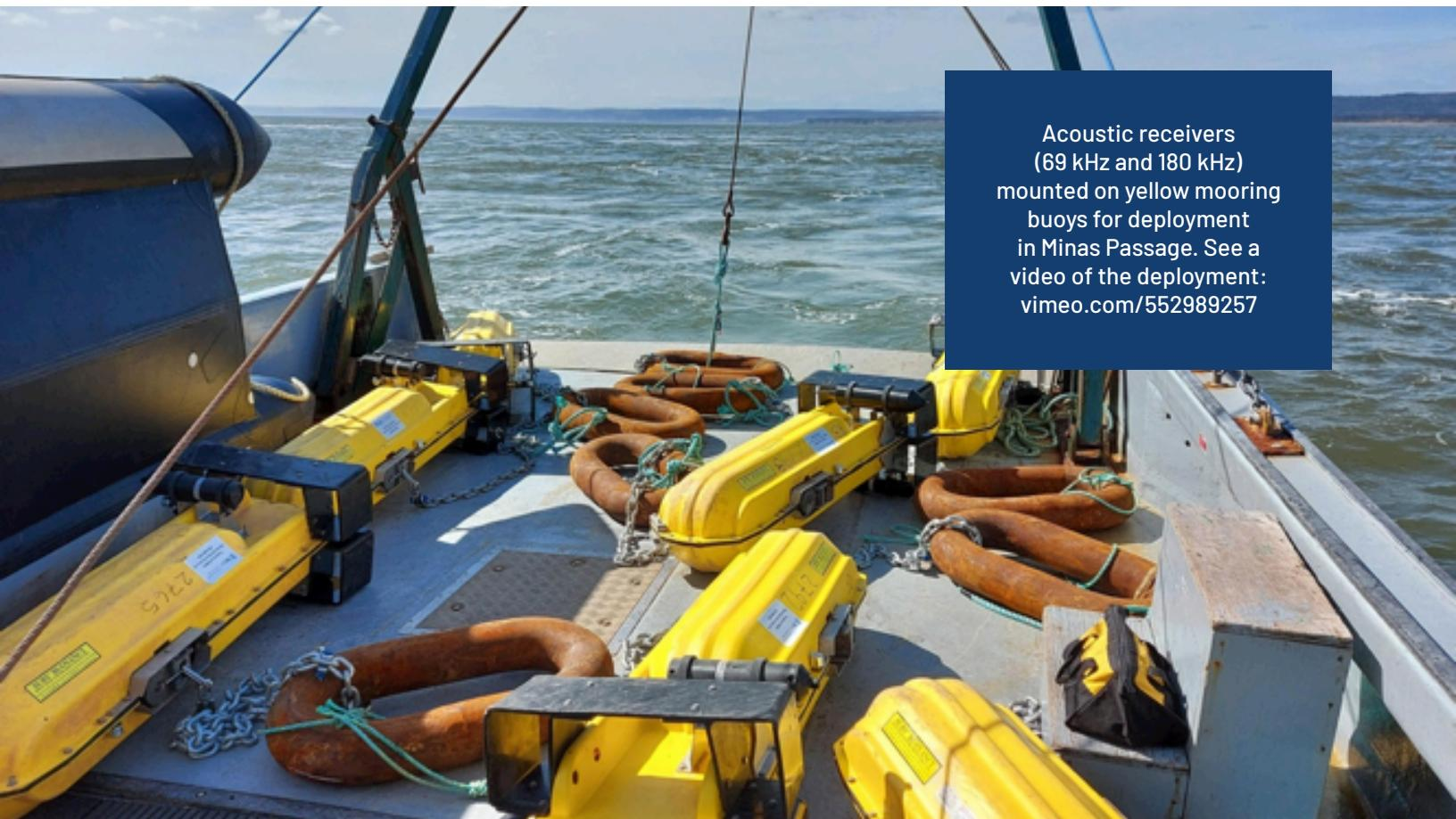
Acoustic receivers (69 kHz and 180 kHz) mounted on yellow mooring buoys for deployment in Minas Passage. See a video of the deployment: [vimeo.com/552989257](https://vimeo.com/552989257)
