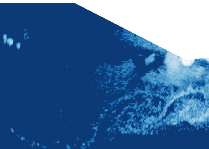
New radar imaging reveals spiralling eddies, in real time, generated during an ebb tide by Cape Sharp in the Minas Passage, Bay of Fundy. Oceanographic features like these can significantly impact the distribution of fish. See time-lapse video of radar data in the Minas Passage: [fundyforcelive.ca/#!/radar](http://fundyforcelive.ca/#!/radar)
